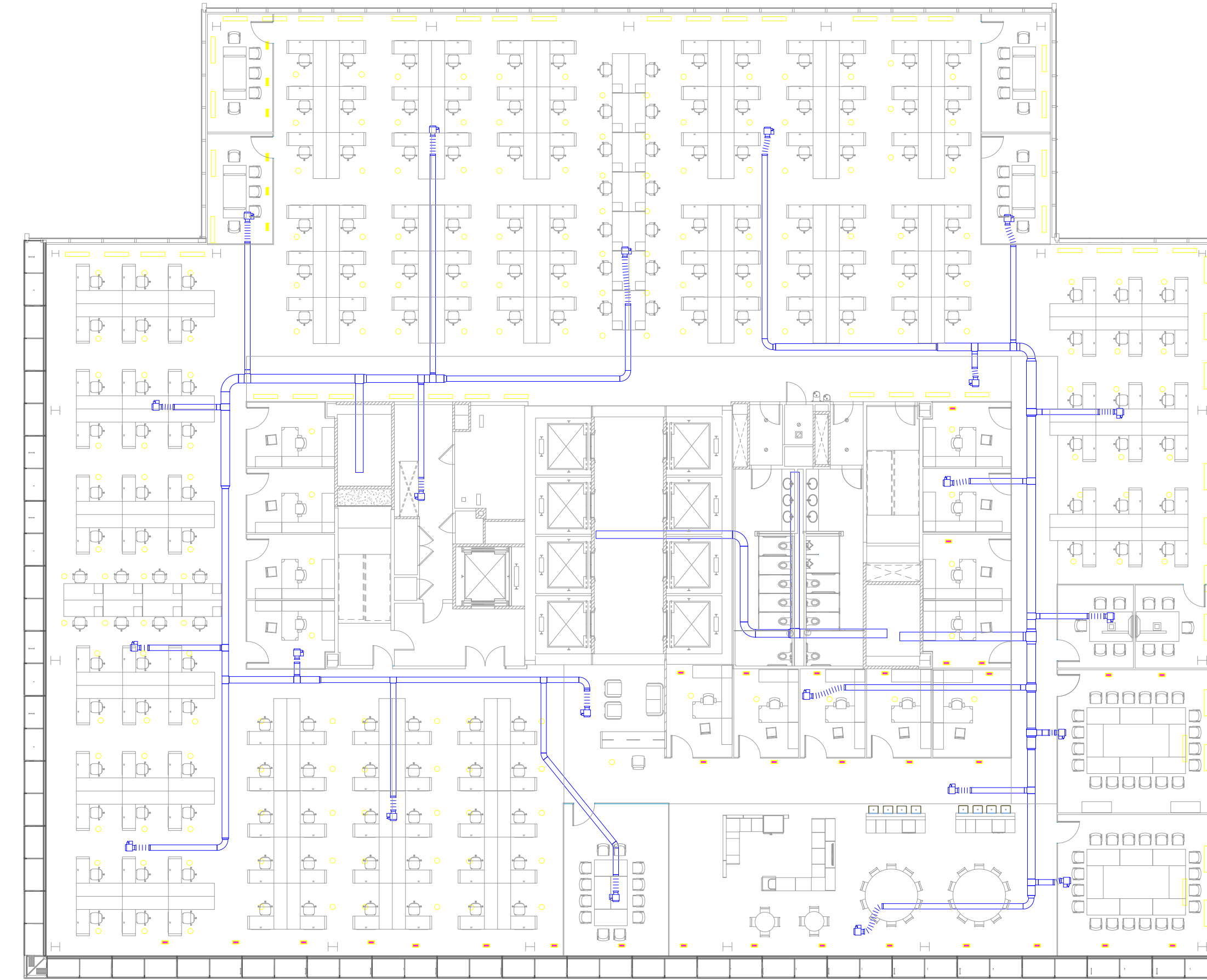
MECHANICAL DIFFUSERS AND RETURN DUCTS PLAN
